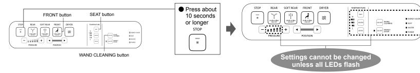
All LEDs on the control panel flash.
