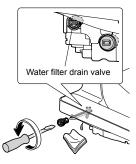
(4)Drain the water from the water supply hose. (Expext Concealed power connection type)
