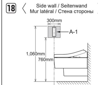
**19** Temporarily place the remote control in the position determined in 18 and confirm the signal reception of A-1.
