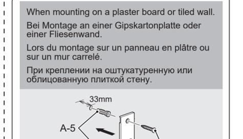
**When mounting on a plaster board or tiled wall.**
